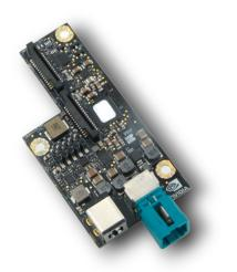
To be able to capture the ZED X on NVIDIA Jetson AGX platform, one of the solution is to use the GMSL2 capture card that connects directly to the CSI port of the Jetson.
